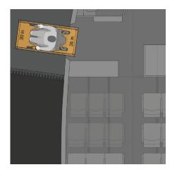
FIGURE 4-9 Forward boarding door clearances, Boeing 737.
