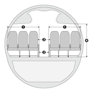
FIGURE 2-8 Cross-section of narrow-body cabin interior with six-abreast seating. NOTES: Dimension ranges for numbered areas in the figure are illustrative and apply only to common economy cabin configurations for a narrow body:
