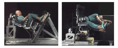
FIGURE 3-1 Dynamic tests (vertical [14 g] and longitudinal [16 g]) to demonstrate compliance with § 25.562.
