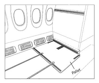
FIGURE 2-9 Aluminum pallet for distributing load across airplane floor structure. SOURCE: European Patent Application.<sup>17</sup>
