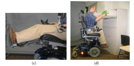
FIGURE 2-2 Illustrations of power wheelchair seating functions, including (a) back support recline, (b) tilt seating, (c) leg elevation, and (d) seat elevation. SOURCE: Human Engineering Research Laboratories, University of Pittsburgh.
