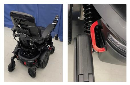
FIGURE 2-5 Power wheelchair with four securement points (red) required by WC19 for a four-point WTORS. SOURCE: University of Michigan Transportation Research Institute.
