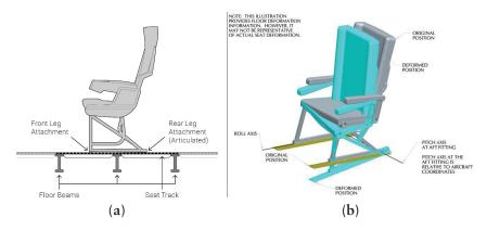
FIGURE 3-2 Illustrations of (a) a typical economy class passenger seat assembly and attachment to seat track, and (b) the floor and seat deformation position. SOURCE: (b) SAE International.
