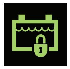
FIGURE 3-5 Label indicating compatibility of battery with RESNA WC25 standards. SOURCE: RESNA.
